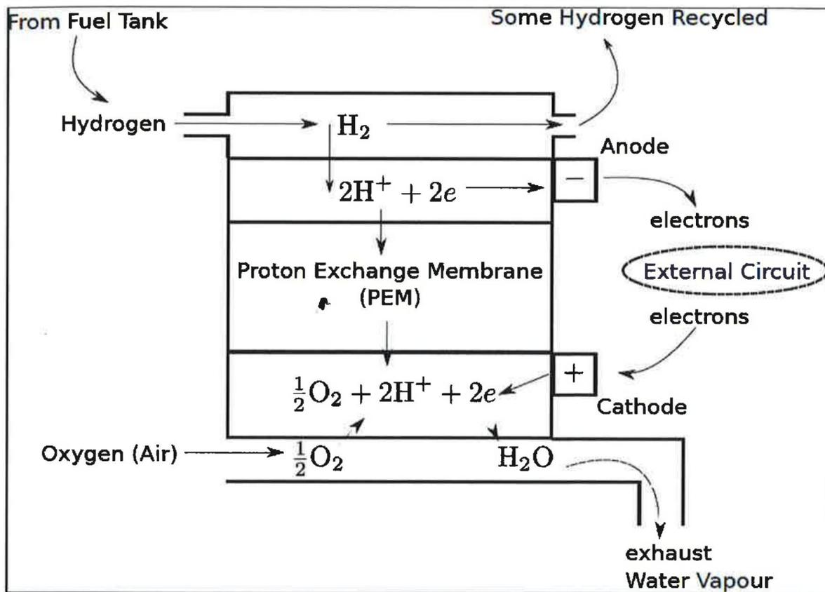
Under the acidic conditions, shown in the diagram, the water is produced at the cathode and hydrogen ions at the anode:
